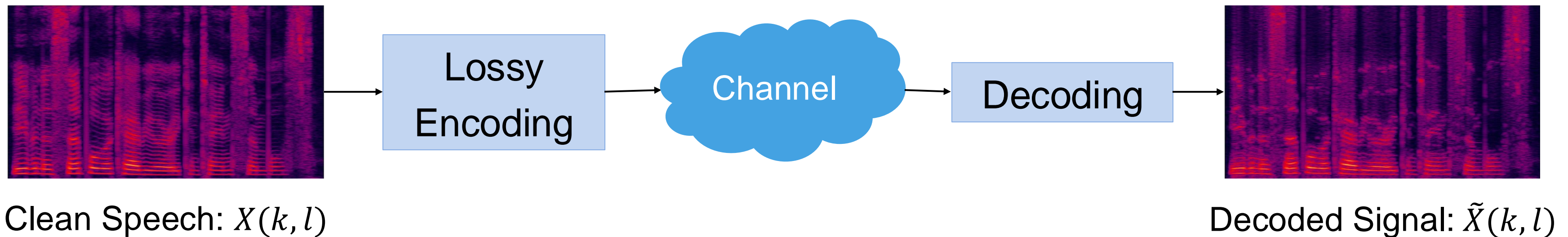
Fig. 1. Lossy codec framework
